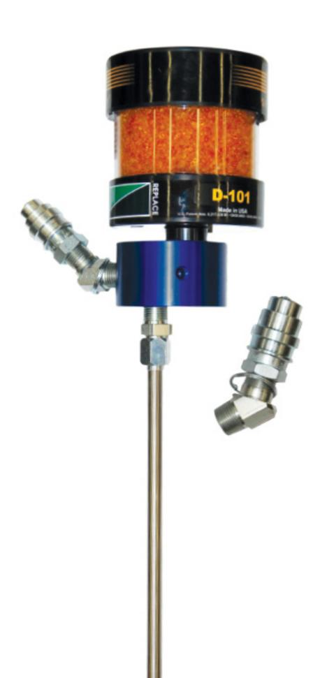
Our Hydraulic Adapter Kit allows you to easily adapt your equipment with a desiccant breather and quick connects with the use of a 6-hole adapter. This allows your system to remain completely sealed to atmospheric ingression, while allowing for easy access during offline filtration or topping reservoirs off.
