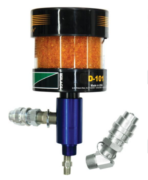
Our Gearbox Adapter Kit allows you to easily adapt your equipment with a desiccant breather and quick connects with the use of a ¾" NPT threaded adapter. This allows your system to remain completely sealed to atmospheric ingression, while allowing for easy access during offline filtration or topping reservoirs off.
